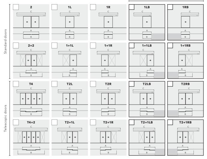
A: Width of the Passage Size | B: Width of the wall opening | C: Length of the Supporting Profile
